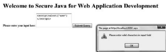
Figure 10.5 JavaScript validation used to prevent the entry of special characters in the input field.
